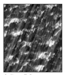
Ordinary Teflon tape Voids clearly visible as splotches. This tape was 86% void by volume.
