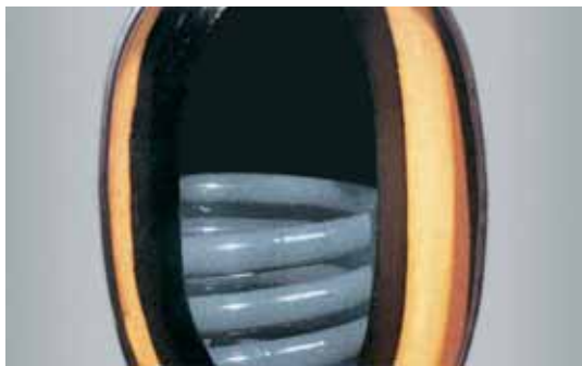
Detail of the heat exchanger
